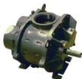
Gears are installed on the end of each shaft to control the position of the impellers, with relation to each other, and thus maintain the clearances needed to assure maximum air flow efficiency, minimum wear, and long life. Since there is no contact between the impellers and the inside of the blower, internal lubrication is not needed and water sealing is not required. In fact, the blower is not able to handle liquids.
